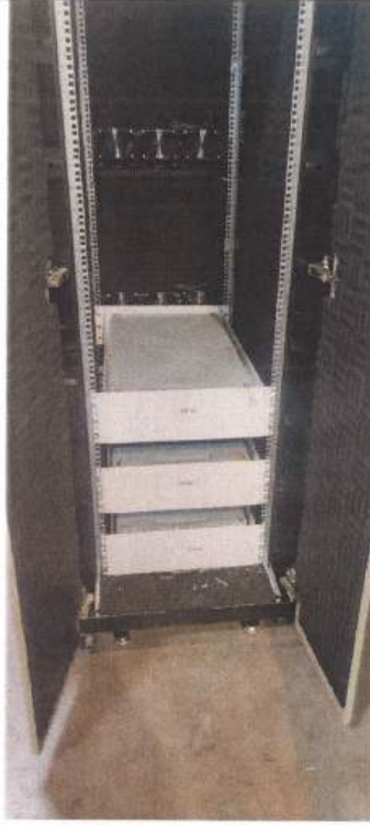
42U (W=750X,D=1130XH=2110) Cabinet dynamic load test
