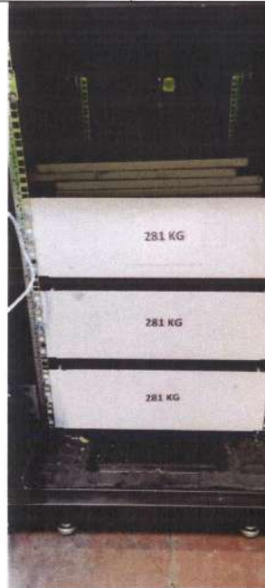
17 U (W=750X,D=1130x H=1000) Cabinet static load test
