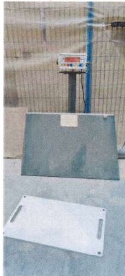
Each weight used for testing 32.2 kg
