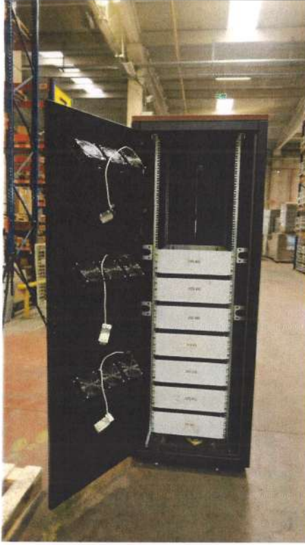
42U (W=750X,D=1130XH=2110) Cabinet static load test
