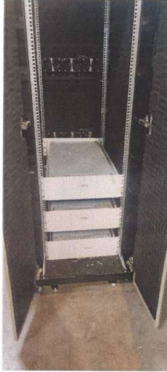
42U (W=750X,D=1130XH=2110) Cabinet dynamic load test
