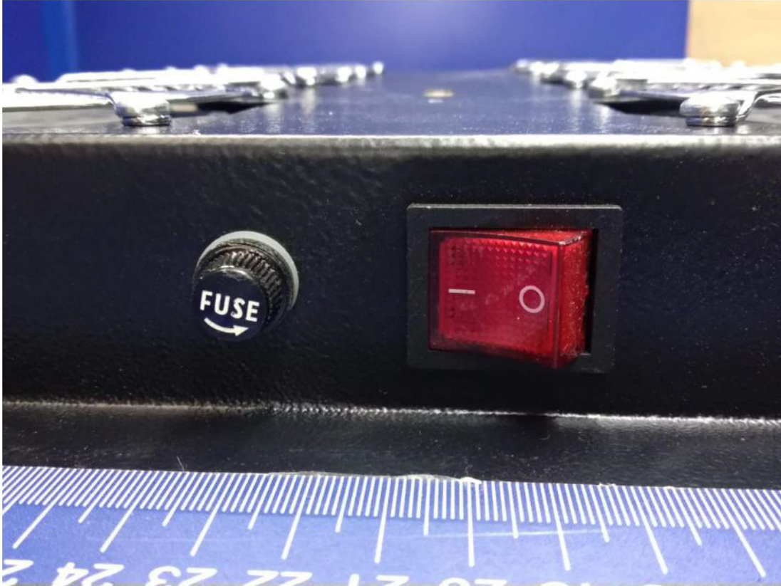
Photograph 3: Fuse holder and on/off switch
