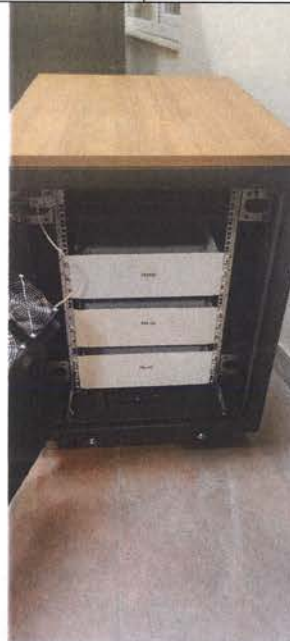
17 U (W=750X,D=1130x H=1000) Cabinet dynamic load test
