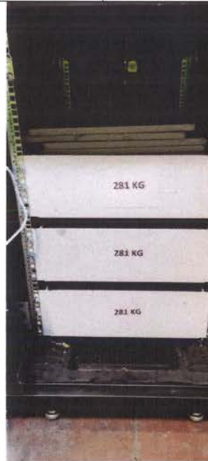
17 U (W=750X,D=1130x H=1000) Cabinet static load test
