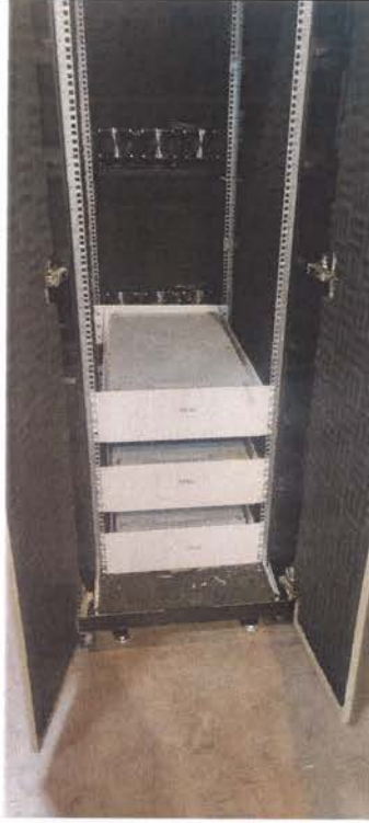
42U (W=750X,D=1130XH=2110) Cabinet dynamic load test
