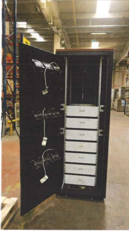
42U (W=750X,D=1130XH=2110) Cabinet static load test
