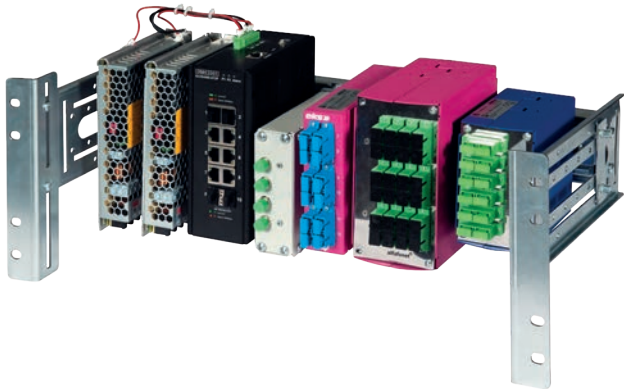
4U DIN rail depth/height adjustable, 4U and 2U 19" connection bars included, t=1,5 mm zinc plated steel, with rear cable management tire, up panel structure. In standard delivered with both 2U and 4U connection bars. If different height devices installed, with help of 4U brackets, you can allign the different height of equipments on the DIN rail.
